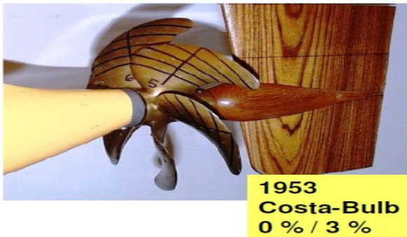
Fig. 2(c): improved propeller design
