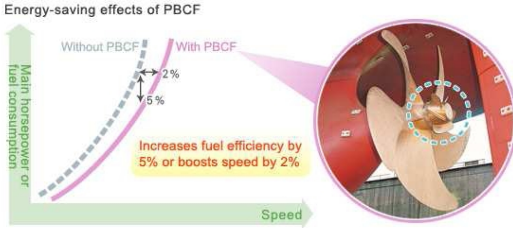
Fig. 7 – Comparison Propellers with and without PBCF
