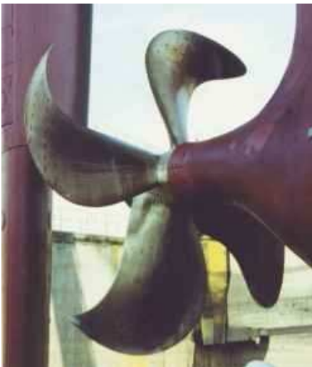
Fig. 8 - The illustration above shows the 14 tonne Kappel propeller unit fitted to the “Nordamerika” of Norden A/S just prior to trials that demonstrated savings of 4%.
