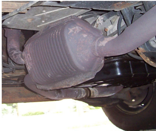
Fig. Catalytic converter on a 1996 Dodge Ram Van (2004)
