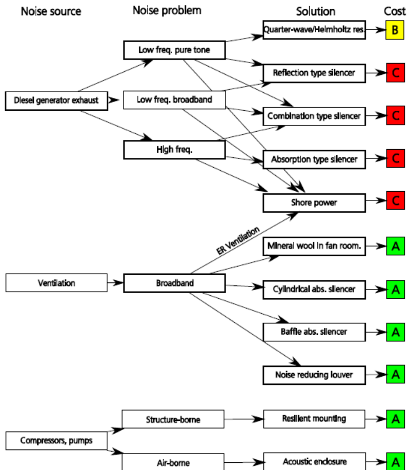
FIGURE: DIAGRAM OF DIFFERENT SOLUTIONS TO DIFFERENT EXTERNAL NOISE PROBLEMS AND THE APPROXIMATED COST OF THE SOLUTIONS. RED COLOUR AND THE LETTER C INDICATES ESTIMATED HIGHEST COST, YELLOW COLOUR AND THE LETTER B INDICATES ESTIMATED LESS COST AND GREEN COLOUR AND THE LETTER A INDICATES ESTIMATED LEAST COST.
