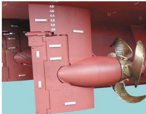
Fig: Efficiency Rudder layout of twin-screw vessel.
