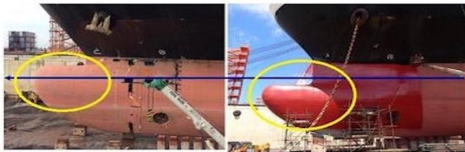
Remodeling of the ship's bulbous bow (Left: Before remodeling) (Right: After remodeling)
