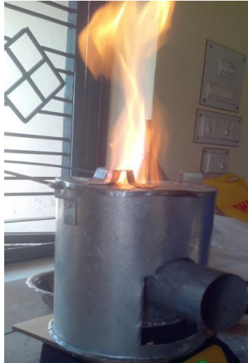
Figure 2: Modified TLUD Stove
