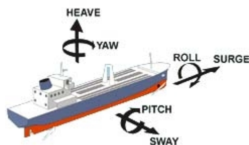
FIGURE NO: 02. MOTION MODEL - FORCES WORKING ON THE SHIP
