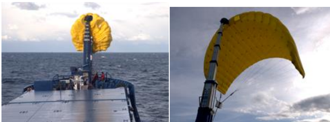
Fig 6: Launch of Towing Kite
