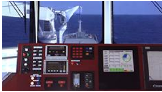
Fig 5: Bridge Control of Launch and Landing of Sky-Sail
