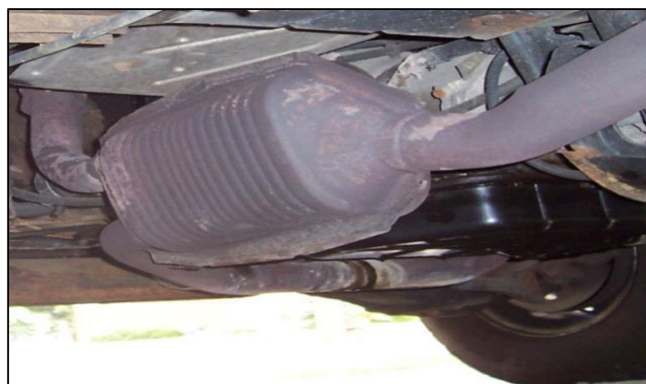
Fig. 4 Catalytic Converter in an Automobile
