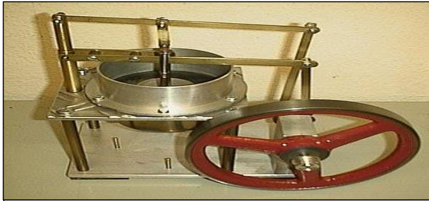
Fig. 1 : The simple working model of Stirling Engine.
