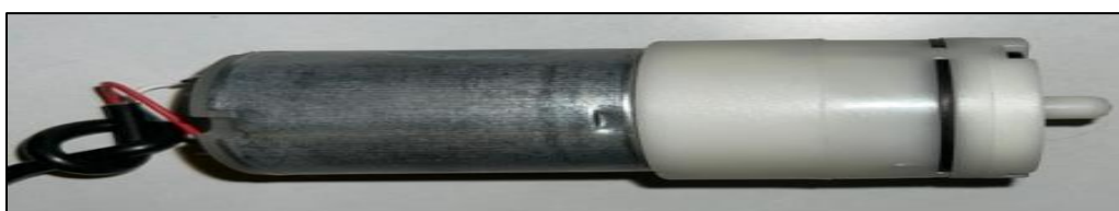
Figure 4:- Compressor coupled with a 12 volts DC motor.
