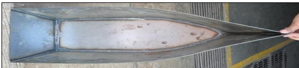
Figure 3:- Mild steel ship model
