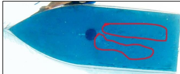
Fig. 7: The Rate of The Air Inlet Is Too Less And Hence The Microbubbles Aren't Created.
