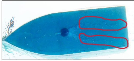
Fig. 6: Bubbles Separated To Near The Hull.
