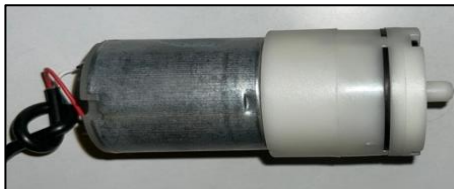
Fig. 4: Compressor Coupled With a 12 Volts DC Motor.
