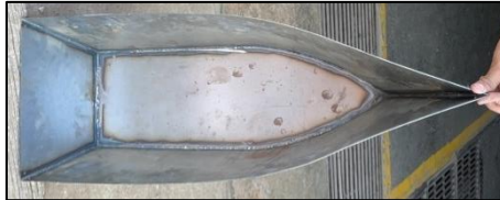
Fig. 3: Mild Steel Ship m\|Model
