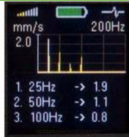
FFT spectrum with peaks detection
