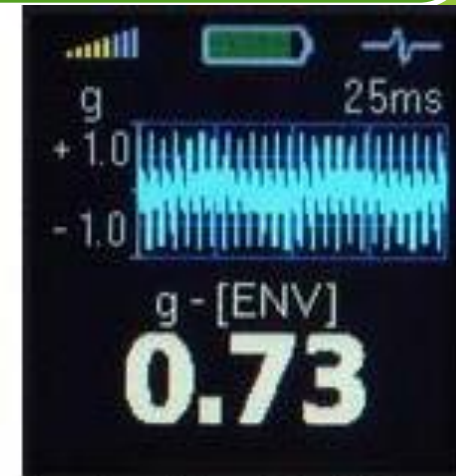
Acc time signal for bearing condition
