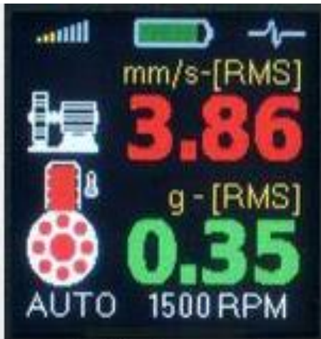
RMS values and temperature of bearing
