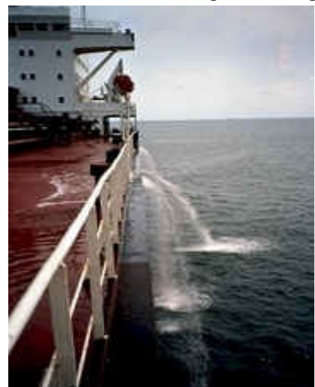
Figure 1: A cargo ship pumps ballast water over the side
