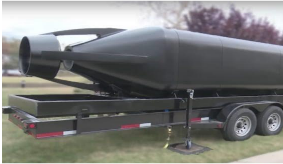
Fig Picture of 3D printed submarine hull prototype by the U.S. Navy
