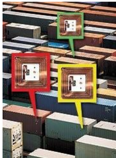
RFID tags attached to containers for easy identification
