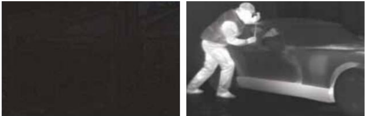
FIGURE 5. Normal CCTV Footage and Thermal Infrared Vision Camera Footage.
