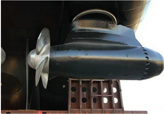
The CRP azipod propeller design
