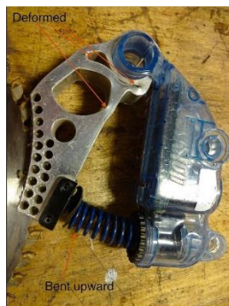
Figure 4.2.2.2.1 SawStop's Braking System
